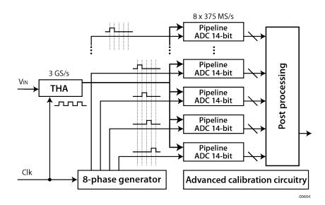
Ridgetop's time-interleaved ADC architecture; IP sub-blocks are also available
