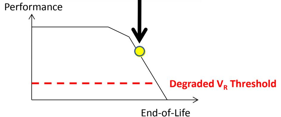
Both supplies provide regulated voltage, but one is degraded and will soon fail.
