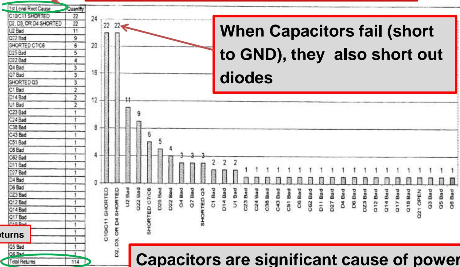
When Capacitors fail (short to GND), they also short out diodes
