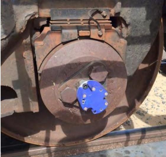
Fig. 1. RotoSense module mounted on the hub of a boxcar axle.
