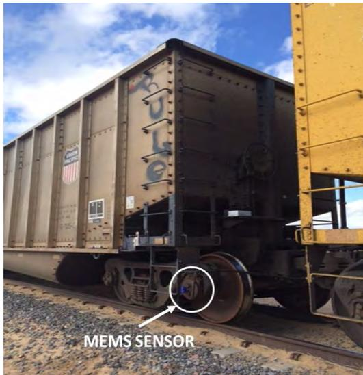
Fig. 12. RotoSense sensor is mounted on the wheel of trailing axle of the trailing truck.
