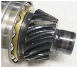
Figure 8. Failed gear – fractured tooth
