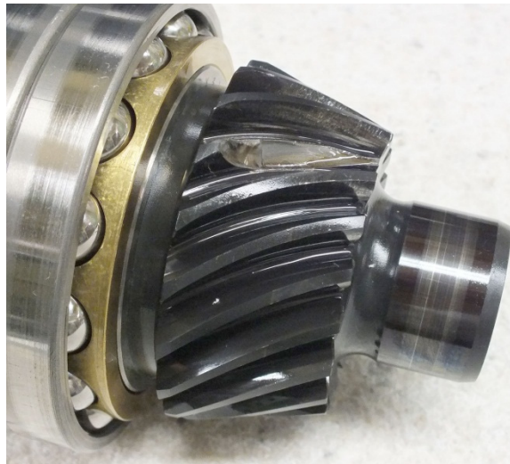
Figure 11.—Fractured spiral-bevel pinion tooth after 112.36 hr run time.
