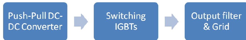
Figure 7: Inverter subsystems, operating serially
