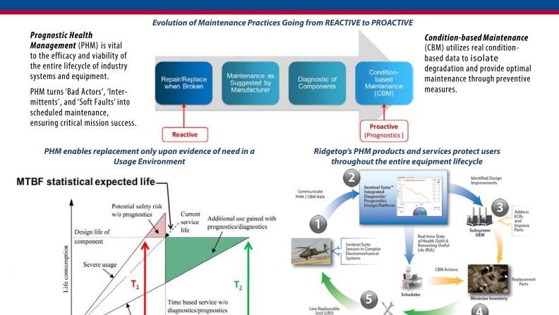
Integration of sensor arrays that identify, isolate and diagnose degradation and communicate SoH and RUL through the Sentinel Suite™ platform Reassess system in real-time to schedule maintenance optimally, saving lifetime costs, reducing labor hours, and increasing part quality
