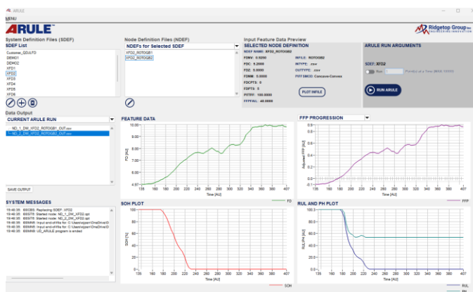
Figure 11: GUI View for Adaptive Remaining Useful Life Estimation (ARULE) software for determining SoH, RUL, and PH from feature data extracted from RotoSense.
