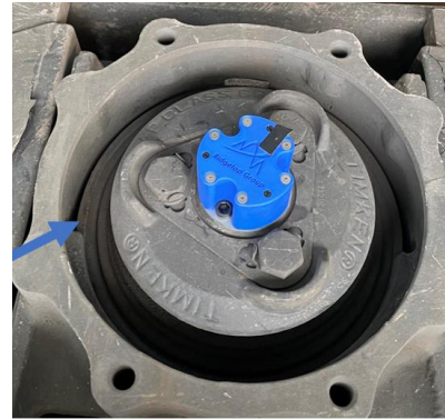
Figure 1: Mounting location of wireless smart sensor when installed on a Timken Bearing end cap.
