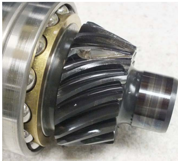
Fig. 11. Fractured spiral-bevel pinion tooth after 112.36 hrs run time.
