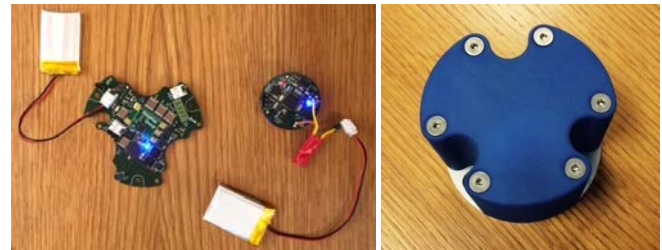
Figure 5. Boards with batteries and housing assembly
