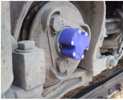
Figure 10: MEMS sensor mounted on a wheel hub
