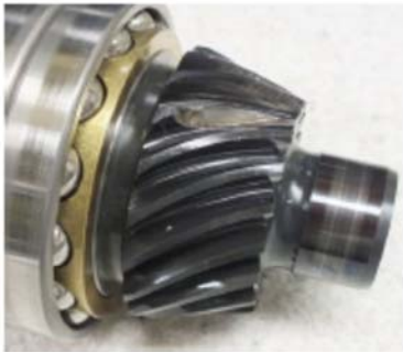
Figure 8. Failed gear – fractured tooth.
