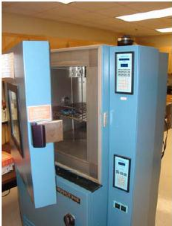
Figure 18: Thermal Oven for Solder Joint HALT Testing – CAVE, Auburn University, Alabama.
