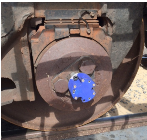
RailSafe RotoSense sensor module (blue) mounted on railcar axle hub
